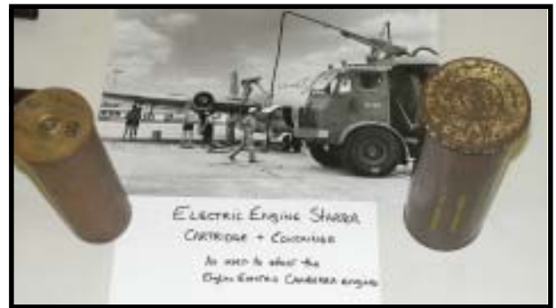
Starter cartridges for English Electric engines in the Canberra bombers
