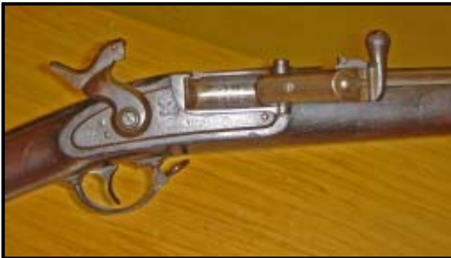
Needhams Patent conversion of the Springfield Musket. An unusual exhibit in this part of the world. A fascinating story surrounds these breechloader. Members should refer to Flayderman's Guide to Antique American Firearms.
