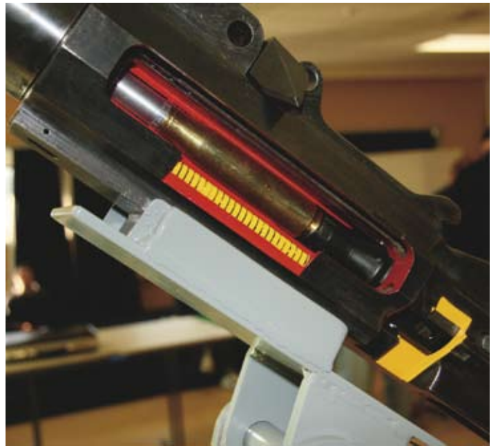
Oerlikon cutaway chamber
