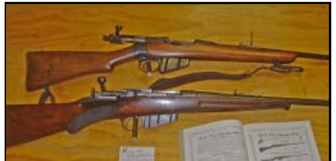
Hunting Rifles. Lee-Enfield and Remington-Lee rifles in .303cal offered by BSA. Note the Lee-Diss magazine on the lower rifle.
