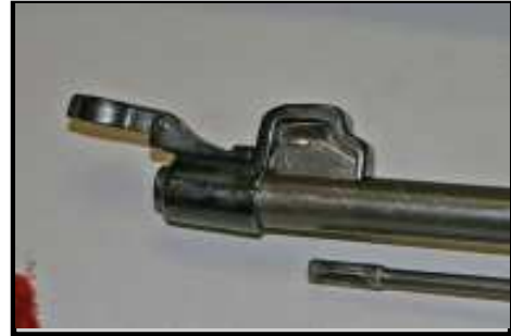
The original foresight and muzzle protector on the above Military Mauser. The clearing rod is also visible.
